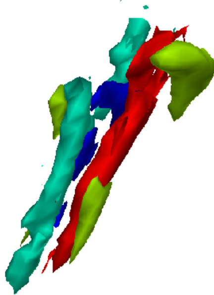
Figure 6. Quasi-streamwise counterrotating vortices together with ejections and sweeps. Quasi-streamwise vortices extend for about 200 – 300 wall units. Two isosurfaces of the same absolute value of \Omega indicate clockwise rotating (red) and counterclockwise rotating (pale blue) vortices. Sweeps and ejections are indicated by green and blue respectively. A time-sequence animation of the events shown in this Figure may be retrieved at http://158.110.50.22/turbulent/movie2.htm
