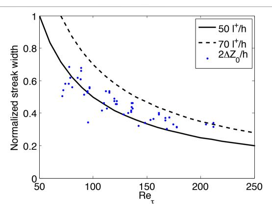
• The width of the streaks is of the same order as the turbulent low velocity structures near the wall.
