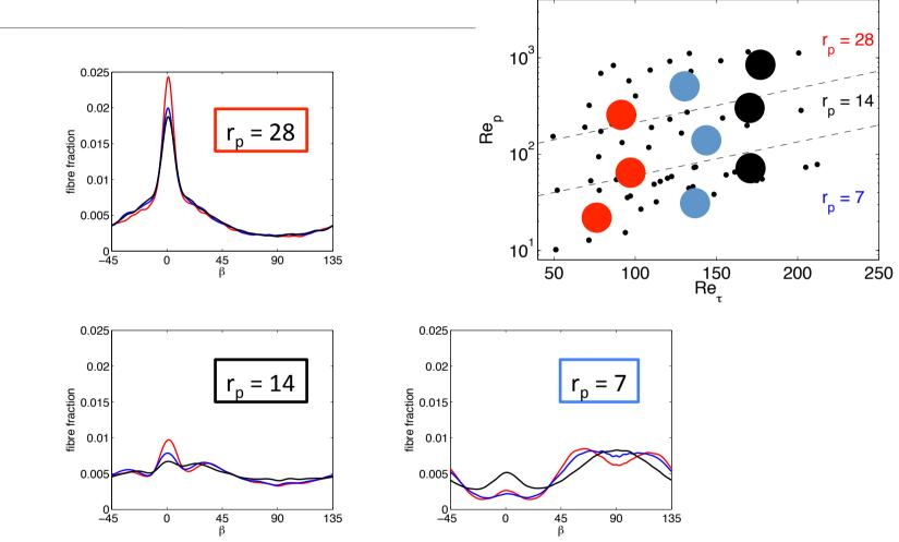
• Fibre orientation depends heavily on fibre length.
