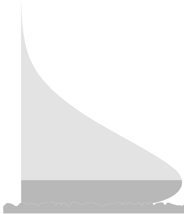
Effects of roughness on the inner layer
