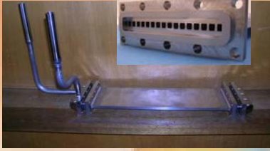
Cooling Plate Mock-up ready for testing
