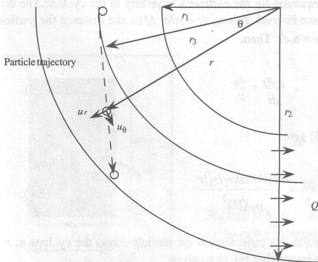
**Figure 8.2** Trajectory of a particle in laminar cyclonic flow
