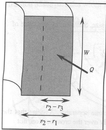
Figure 8.3 Schematic diagram of a cyclone entrance channel
