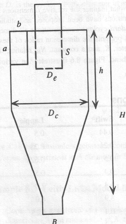
Figure 8.6 Dimensions of a standard cyclone
