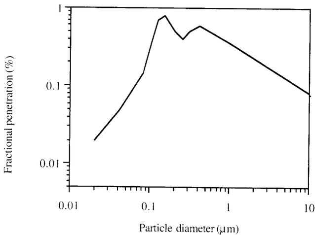
**Figure 10.2** Measured baghouse fractional penetration (From Carr, R. C., and Smith, W. B. *JAPCA*, 34:79, 1984; reprinted with permission from *JAPCA*)
