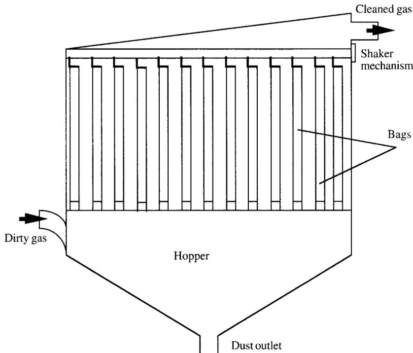
**Figure 10.1** Schematic diagram of a shaker baghouse
