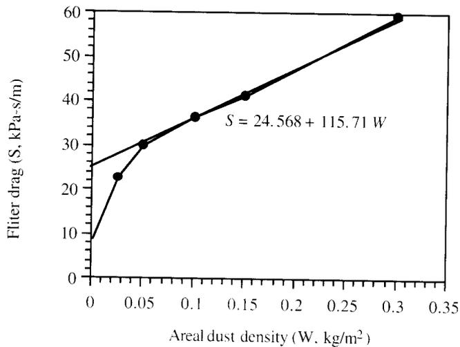
**Figure 10.4** Filter drag versus dust areal density for Example 10.2
