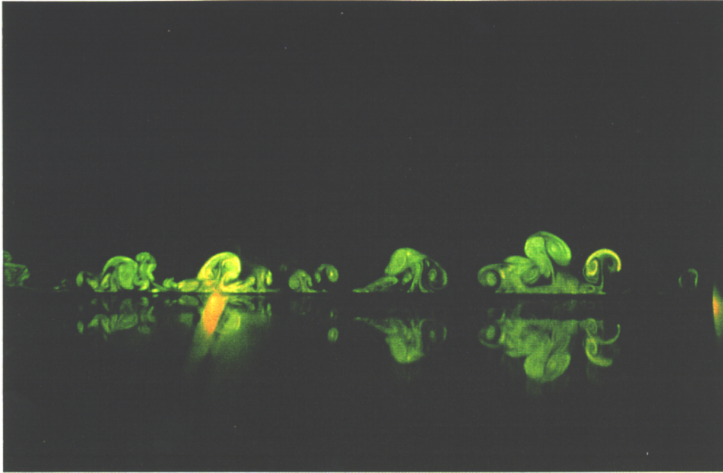
Figure 5 LIF view looking upstream, sheet perpendicular to both plate and free stream, located 8.3 plate thicknesses downstream of separation. Reynolds number based on plate thickness is 890.
