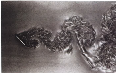
172. Wake of an inclined flat plate. The wake behind a plate at 45^\circ angle of attack is turbulent at a Reynolds number of 4300. Aluminum flakes suspended in water show its characteristic sinuous form. Cantwell 1981. Reproduced, with permission, from the Annual Review of Fluid Mechanics, Volume 13. © 1981 by Annual Reviews Inc.
