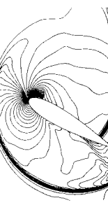
Fig. 18.13. Density contours for the shock passage past a NACA 0018 aerofoil at 30^\circ incidence (after Yee, 1986)
