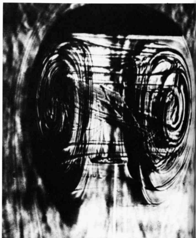
183. Bubble rising in a non-Newtonian fluid. A bubble of 13 \text{ cm}^3 volume rises at a Reynolds number less than 0.1 in a vertical tube of 8.2 cm diameter (not visible) filled with a 3.5 per cent aqueous solution of polyethylene oxide. This fluid possesses both a highly shear-thinning viscosity and considerable elasticity. The bubble loses the fore-aft symmetry it would have in a Newtonian fluid, becoming pointed at the rear. Photograph by M. Coutanceau and P. Thizon, in van Wijngaarden & Vossers 1978
