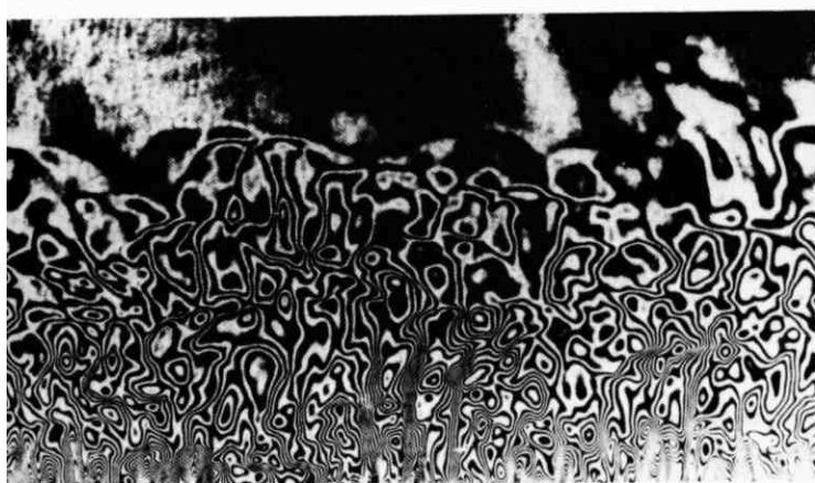
143. Instabilities in a heated layer. Freon between horizontal plates is momentarily heated from below. Successive differential interferograms show instabilities in the starting
