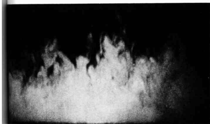
163. Oblique transverse sections of a turbulent boundary layer. The flow is viewed head-on, with smoke illuminated by a sheet of light that is inclined 45^\circ downstream from the wall on the left and 45^\circ upstream on the right.
