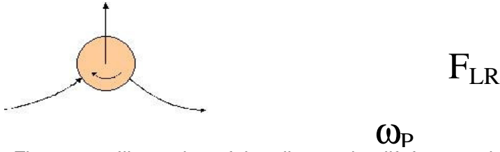
Figure 3.9: Illustration of the slip-rotation lift force acting on a stationary particle
