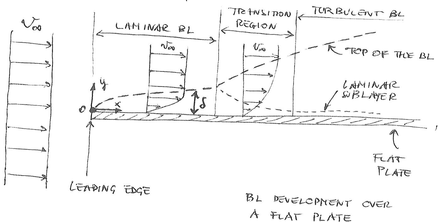
Development of the BL begins at the plate's leading edge ( $x=0$ ): downstream of the leading edge, the flow inside the BL is laminar, for
