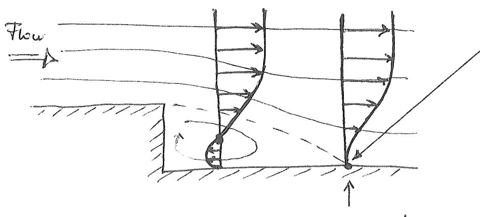
Experiments show that maximum heat flux occurs here, where  $\frac{\partial V_x}{\partial y} \approx 0$  and therefore :
