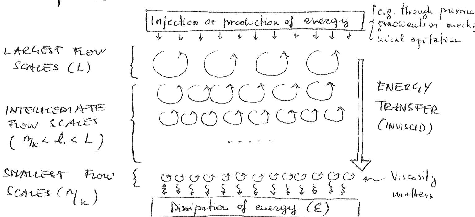
To better explain the physical meaning of energy dissipation rate (without providing a formal mathematical definition), consider a situation in which energy is fed into the flow at scale  $L$ . The Kolmogorov theory assumes that the eddies of size  $L$  become unstable within a time of the order of their TURNOVER TIME  $T_L$ : After this time, eddies of size  $L$  transfer an amount  $\Delta u_L^2$  of energy (per unit mass) to the smaller eddies.
